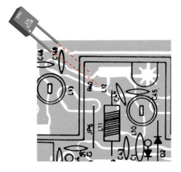
3) Add 68pF capacitor across C42. Install on solder side of PCB. Leave C42 alone.
