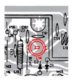
Remove TR14 (the 2SC2078), and install EKL Components' ERF-2030 in its place with stock insulator, washer, and screw.
