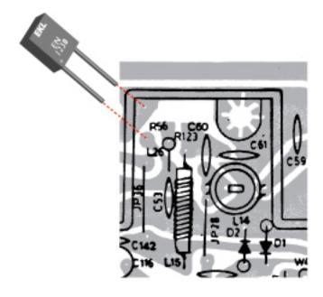
Add 68pF capacitor on back of C59. Install on solder side of PCB. Leave C59 capacitor alone.
