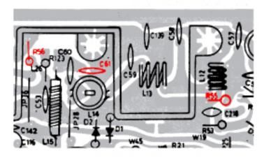
Install EKL Components' EN-1230 at R56. The EN-1230 is a POLARIZED part. Make sure that it is installed correctly with the positive lead toward R123.
